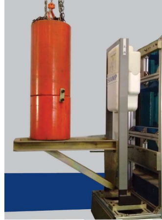
BCU 6030 specification and actual loading test with 400Kg
